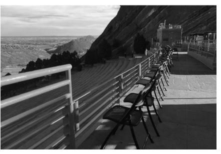
Figure 65 Wheelchair accessible seating in Row 70 at the top of the auditorium has a lowered guardrail to avoid obstructing the view to the stage. 2017.
